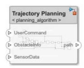
Any change made in a reference architecture is immediately reflected in the models that link to it. If you move or rename the reference architecture, the link becomes invalid and the linked component displays an error. Link the component to a valid reference architecture.
